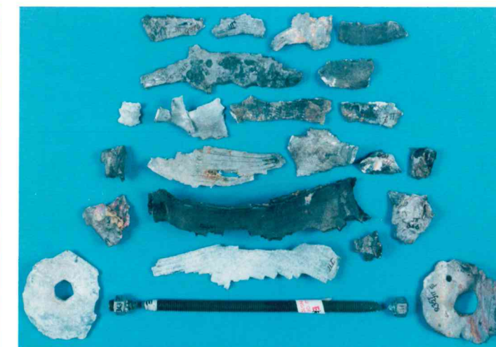
Figure 4. Pipe bomb fragments. This pipe bomb was constructed with a pipe nipple and two welded end plates that formed an enclosure for the explosive.
