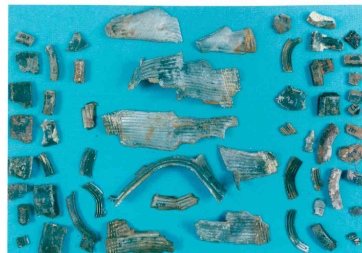
Figure 3. Pipe bomb fragments. This bomb was constructed with a pipe nipple and two threaded end caps to form an enclosure for the explosive.
