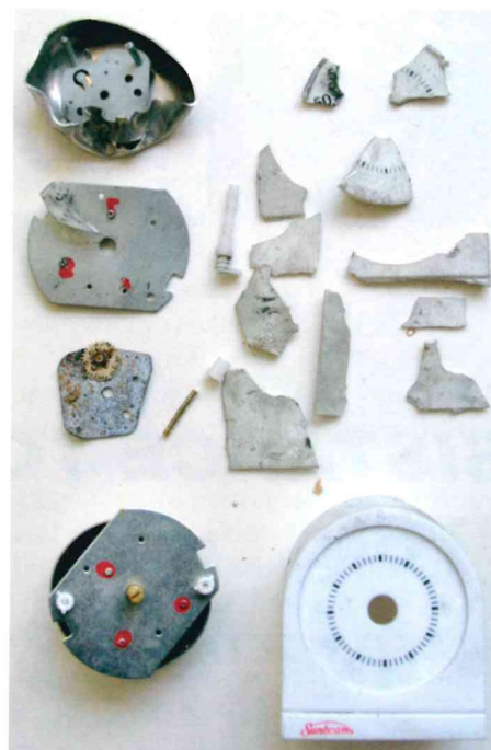
Figure 1. Fragments of a mechanical timing device compared with undamaged components.
