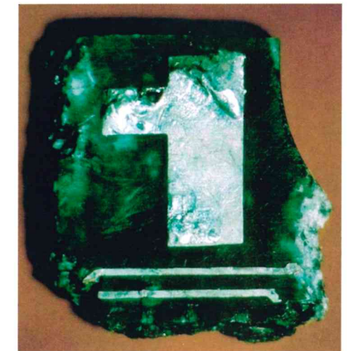
Figure 7. Small section of a circuit board that was part of the MST 13 electronic timer for the bomb that destroyed Pan American Flight 103 over Lockerbie, Scotland in 1988.
