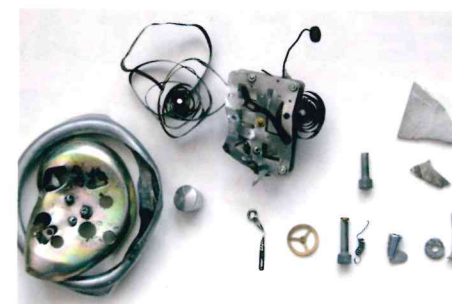
Figure 2. Remains of a mechanical clock used as a timing device, found after a bomb blast.
