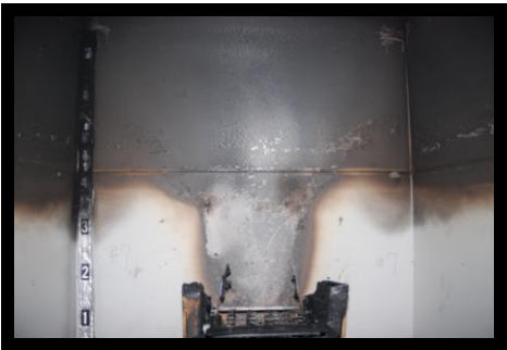
Figure 12: Chair 7 42'' Header - Actual Damage (left); Calcination Measurements (center); Thermocouple Data (right)
