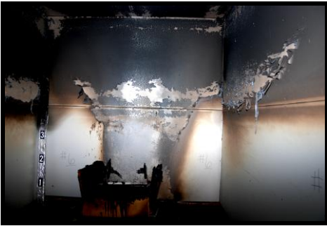
Figure 11: Chair 6 30'' Header - Actual Damage (left); Calcination Measurements (center); Thermocouple Data (right)
