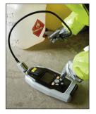
Manufacturer's literature advises that the system is waterproof to one meter submersion, operates in ambient conditions of -20 °C to +40 °C and is rugged as per MIL-STD-810F compliance for drop, shock, and vibration. However, these specifications were not the object of the testing.
