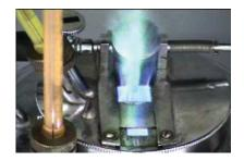
Figure 1: Closed Cup Flash (Paraxylene)
