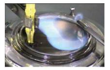
Figure 2: Open Cup Flash (Paraxylene)
