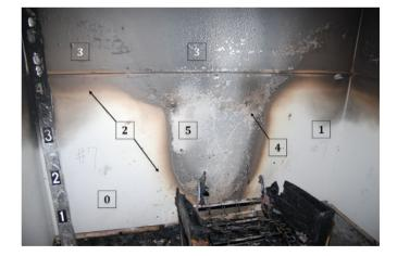
FIG. 1—Photograph from which selected images of visible damage indicators was chosen for use with the DOFD Method.
