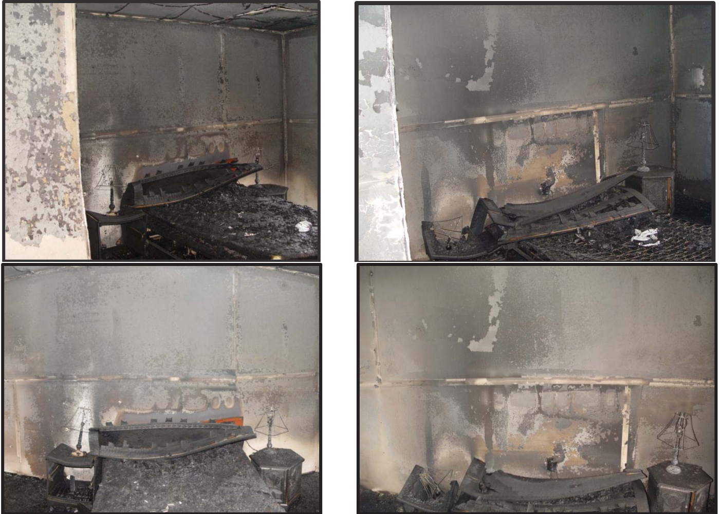
Figure 9: Post-fire Damage-Left Nightstand=Area of Origin (left) Cell 1; (right) Cell 2
