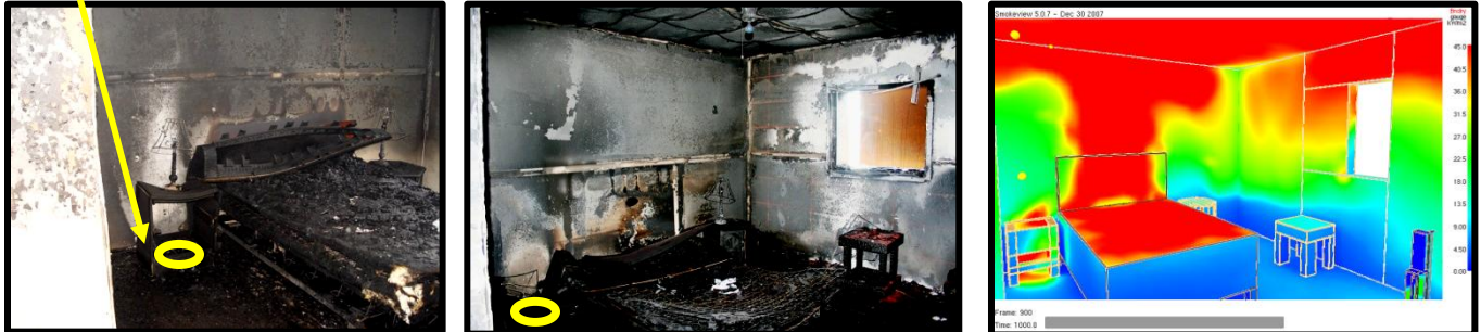
Figure 10: East Wall Actual Damage Cell 1 (left), Cell 2 (middle) versus FDS Heat Flux Calculation (right)
